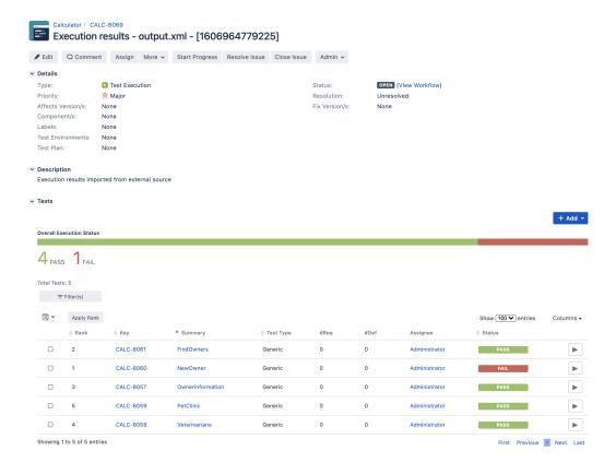
Each model is mapped to JUnit's <testcase> element which in turn is mapped to a Generic Test in Jira, and the **Generic Test Definition** field contains the unique identifier of our test; in this case it's "model.<name\_of\_model>". The summary of each Test issue has the name of the model.
