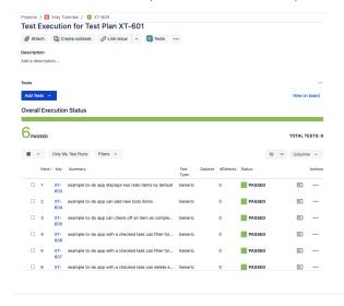
Tests implemented using Cypress will have a corresponding Test entity in Xray. Once results are uploaded, Test issues corresponding to the Cypress tests are auto-provisioned, unless they already exist.
