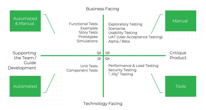
What is clear from this diagram is that Tests can either be manual, automated or you can also use tools to help you perform certain types of tests (e.g. for load testing).
