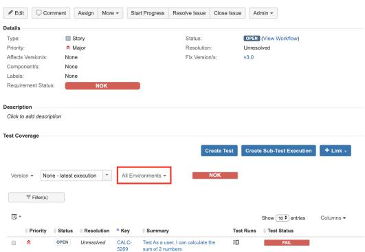
If you want to analyze the coverage for the requirement (e.g. "story") and show the latest results on that environment, just use the picker on the "Test Coverage" section. As seen ahead, this will produce different results because different results were obtained in different environments.
