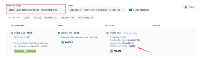
Traceability Report being used to analyze the results of a Story for the "Firefox" Test Environment.
