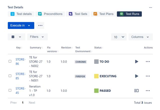
The same test has been executed in both Test Environments (a Test Execution per Test Environment).
