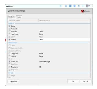
A possible "Valid Login" test case could be composed of a setup section to open the browser (i.e. using the "OpenBrowser" module), a recorded module where we enter the credentials and validate the welcome page, followed by the close browser instruction (as part of the CloseBrowser module).
