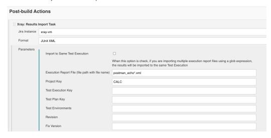
A Test Execution will be created containing results for all tests executed. Actually, in our specific case and only for demonstration purposes, two Test Executions would be created due to the fact that we're generating two JUnit XML files from the different Newman reporters.
