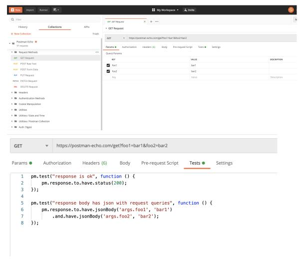
In the previous example, we can see two tests: one for validating a successful HTTP request based on the status code and another that checks the response's JSON content.
