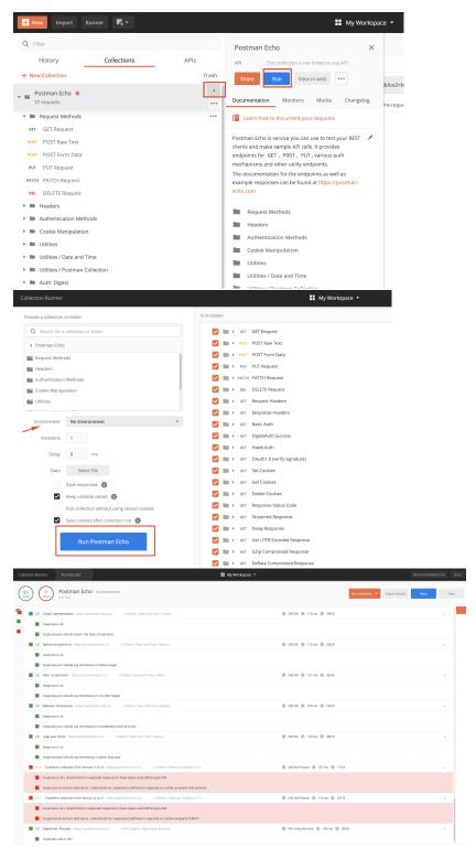
The runner shows the overall count for the number of passed and failed tests. We can also see the assertion error on failed tests; in this case, saving the response (setting the proper flag above) can help us better understand what is happening.
