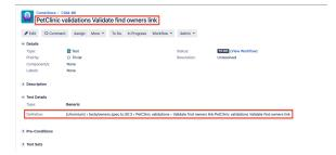
Xray uses a concatenation of the suite name and the test name as the the unique identifier for the test.
